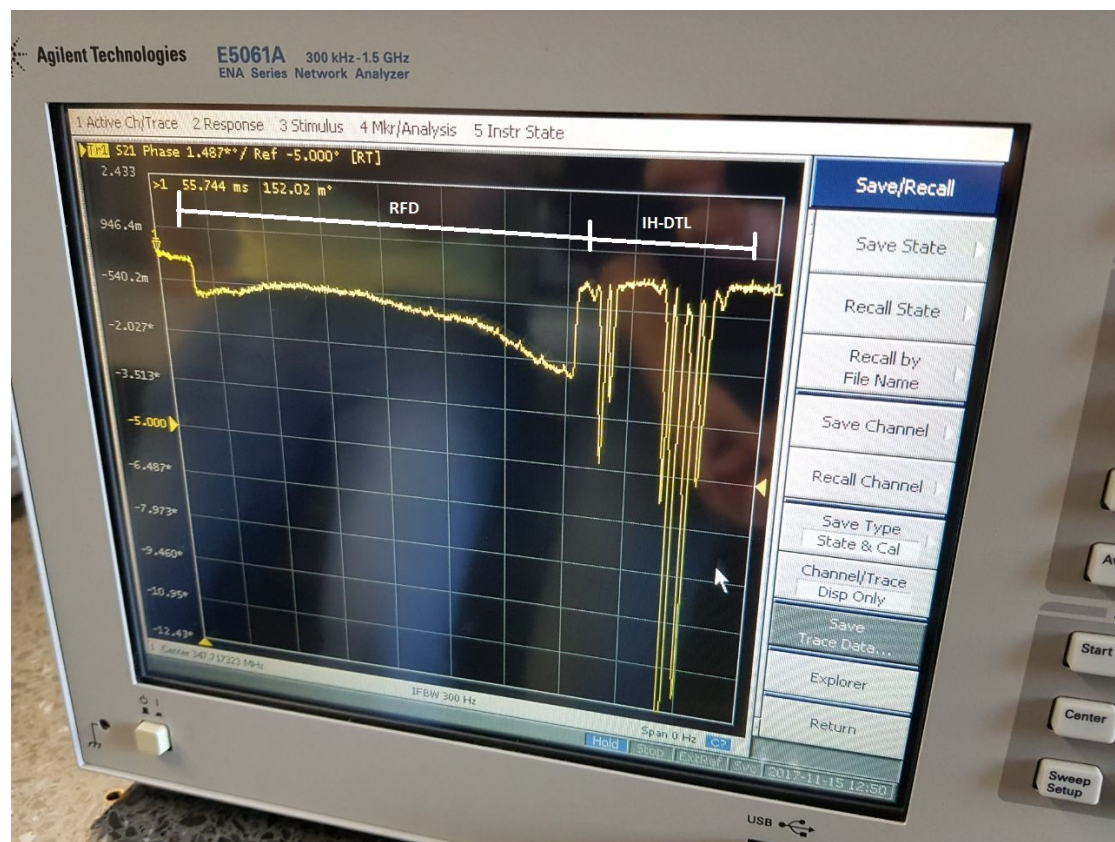
Figure 5: Network analyzer after the bead-pull measurement on the coupled model pressed on the touchscreen of the display.
