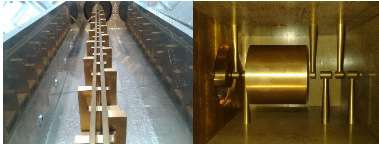
Figure 4: Left: View of the RFD along the beam axis, right: Plan view of the IH-DTL
